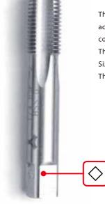
The two-piece set for inner pipe threads according to DIN ISO 228 part 1, consists of taper and bottoming. The taper has undersize. Sizes from G 1/16 to G4 have a reduced shank and four flutes. The pitch is indicated as threads per inch (25,4 mm).
